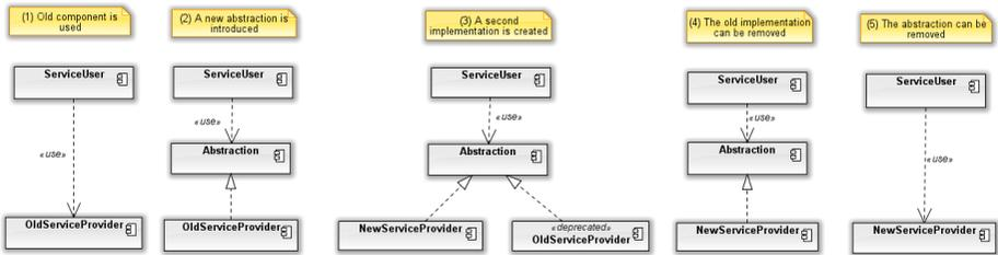
**Fig. 2.** A component is substituted with a new implementation through branch by abstraction.
