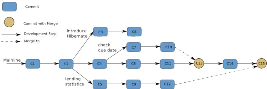
**Fig. 1.** A Repository containing one mainline and three feature branches.
